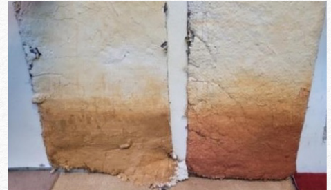
Tango wall sample: plaster on underlay © Valérie Valero
